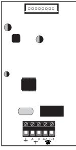
The modem card is used to communicate either via Contact ID, Fast Format, SIA or SMS. It will also enable remote uploading/downloading via a PC to the control panel.
